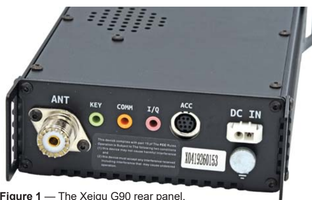
Figure 1 — The Xiegu G90 rear panel.
